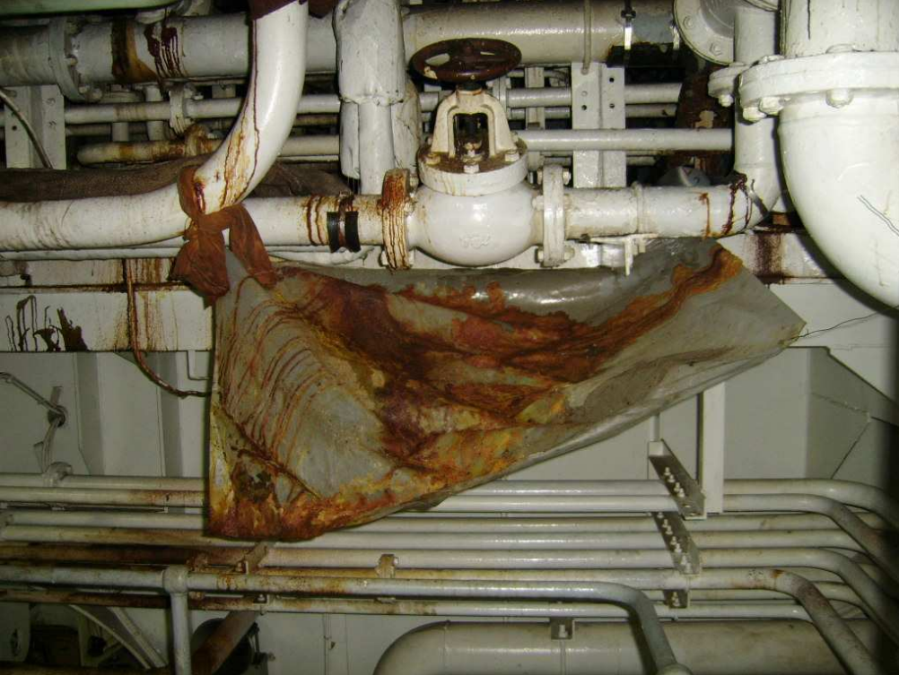
MV Caribbean Mermaid: Numerous temporary repairs at important piping systems in the engine room
